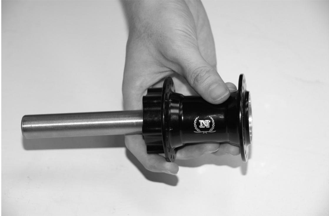
5. Fasten the Expander Tube into hub.
