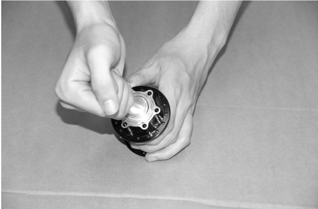
3. Use any tube to take out end cap with rubber O-ring.
