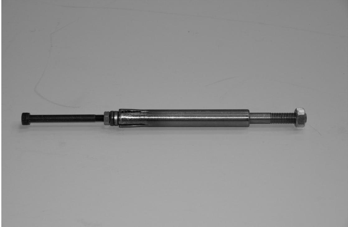
**“Tools 661”** for bearing disassembly.
