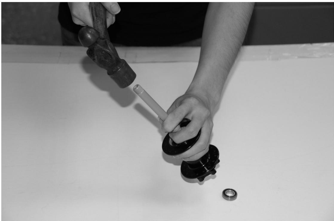
6. Use hammer to tap up the axle to Push farther sealed bearing out.
