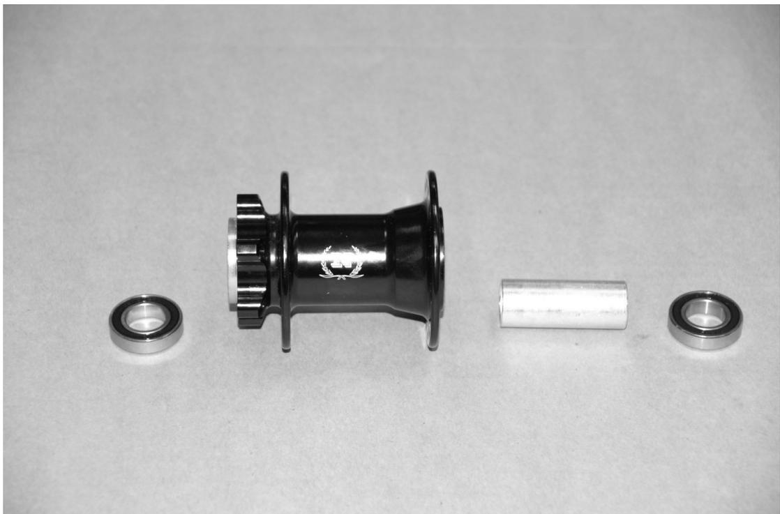
8. After disassemble the parts of hub.
