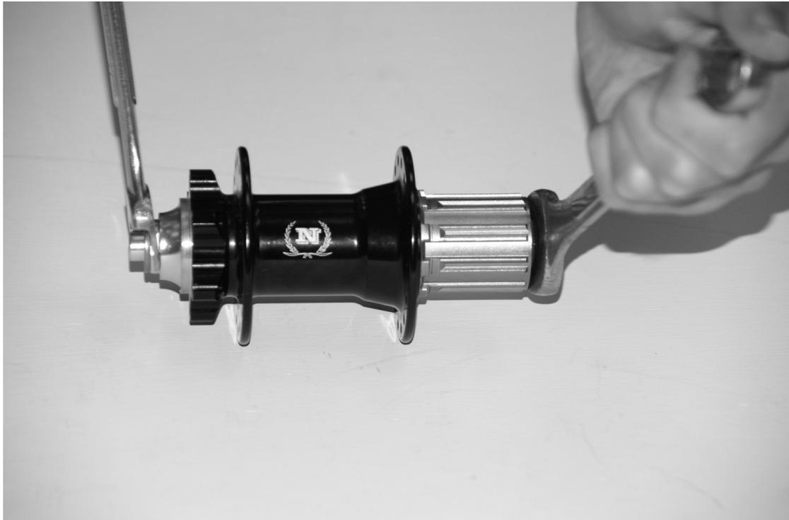
1. Insert two wrench into both side caps and unscrew the side cap.
