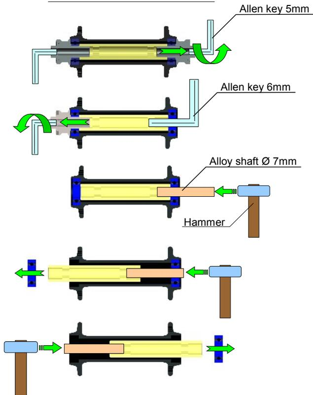
1/ Unscrew right side cap using 5mm allen key in both side caps.
