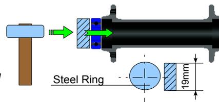
2/ Put axle to hub shell first and bearing near the bearing seat of hub shell.
