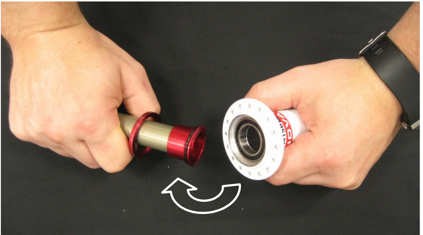
Step 2: Jemmy side cap by 20mm alloy thru axle.
