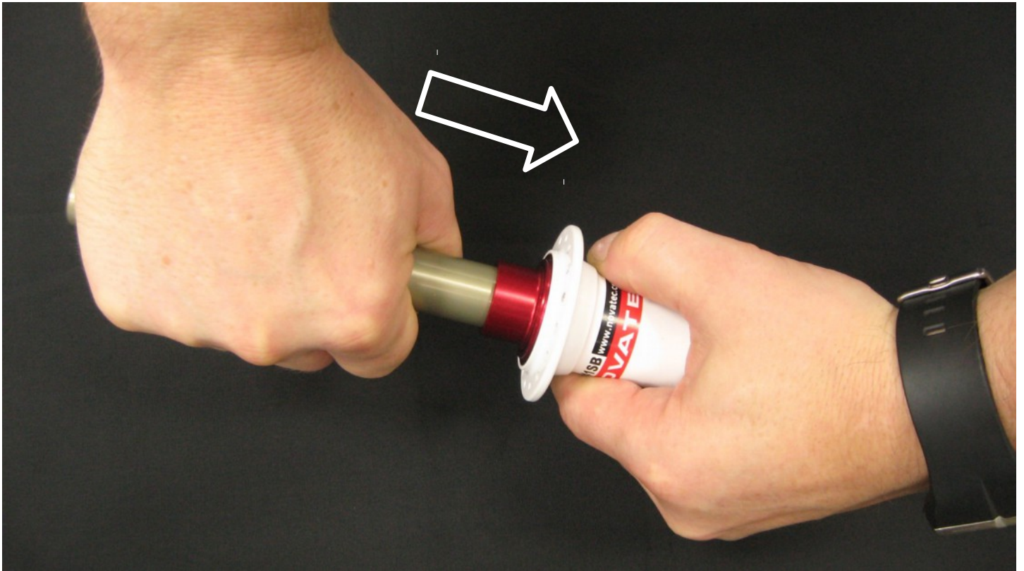
Step 1: Insert 20mm alloy thru axle to side cap.
